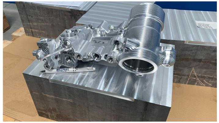
Around half a day of machining and 13.000 measuring points later Millpart has turned the aluminum block into a hydraulic manifold for business jets
